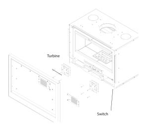
Fig. 2. RK cassette - mounting method of the fans along with the location of switch
