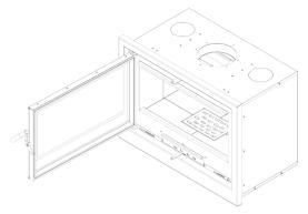
Fig. 9. RK cassette - dismantling the door, step 3
