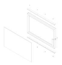
Fig. 6. RK cassette - dismantling the glass
