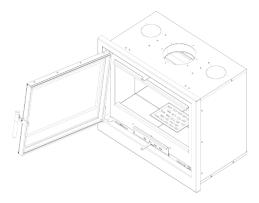
Fig. 11. RK cassette - dismantling the door, step 5
