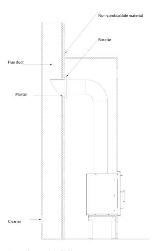
Fig. 4. RK cassette - exemplary connection to the chimney
