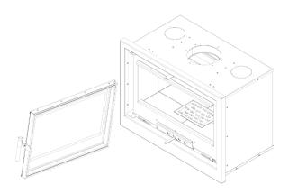
Fig. 12. RK cassette - dismantling the door, step 6
