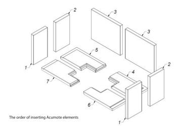
Fig. 14. RK cassette - the order of assembly and disassembly of Acumote components
