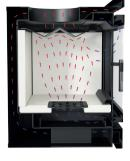
Fig. 1. RK insert - air circulation in the fireplace insert RK
