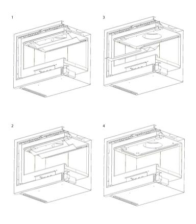
Fig. 13. RK cassette - dismantling the deflector and the slats holding the Acumote
